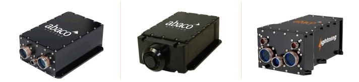
Qualification takes the form of testing for temperature, temperature shock, altitude, humidity, shock/vibration, EMI, sand/ dust, salt spray, water ingress and flammability to standards such as MIL-STD-810G method 514.7, 516.6, DO-160G Sections 4-21, 25 and MIL-STD-561G.
