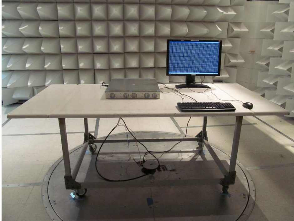
Low Frequency Radiated Emissions Semi-Anechoic Chamber Test Setup, Front View
