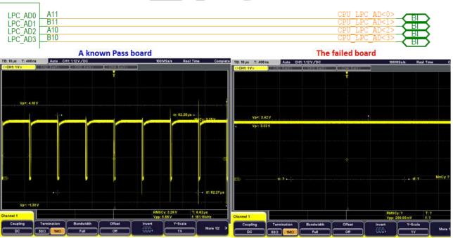
6) Replaced FPGA with a new one, the failure symptom dis-appear
