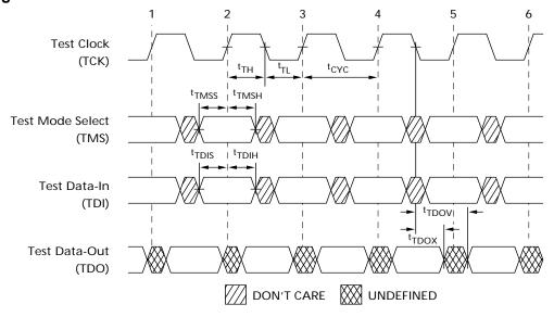
TAP AC Switching Characteristics Over the Operating Range<sup>[10, 11]</sup>
