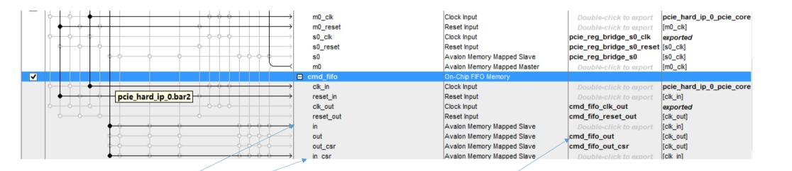
I add a FIFO memory on the basis of Altera PCIR DDR3 reference design IN & IN\_CSR are connected to Bar0/1
