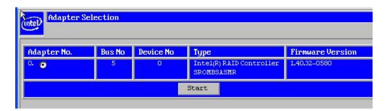
Figure 7 EFI RAID BIOS Console
